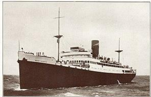
"NOVA SCOTIA" (DUNCAN, WHITE & CO., LTD.) 401 ft. B.P. x 55 ft. 4 in. x 34 ft. 4 in. 6,796 tons gross. 14 knots. 1,150 H.P.
