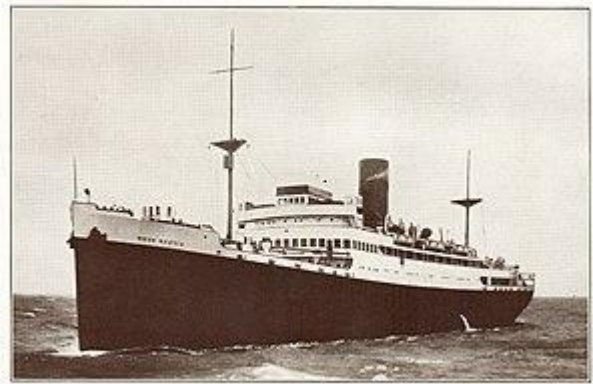
"NOVA SCOTIA" (GARDNER, WHITE & CO., LTD.) 491 ft. B.P. x 51 ft. 1 in. x 34 ft. 4 in. 6,796 gross tons, 14 knots, 5,150 H.P.
